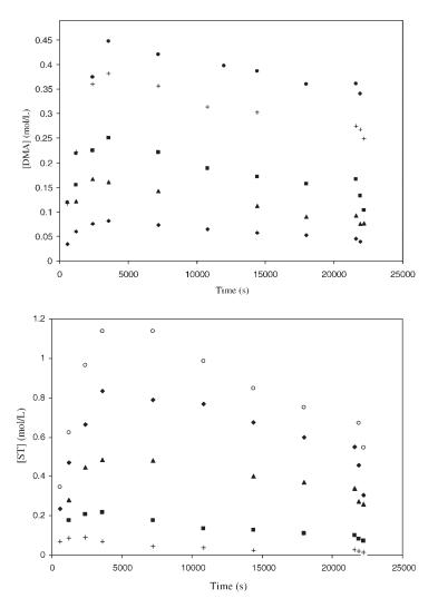
**Figure 1.**[DMA] (top) and [ST] (bottom) semibatch experimental profiles: ST homopolymerization (○); ST/DMA 75/25 copolymerization (♠); ST/DMA 50/50 copolymerization (♠); ST/DMA 25/75 copolymerization (■); ST/DMA 10/90 copolymerization (+); DMA homopolymerization (♠).
