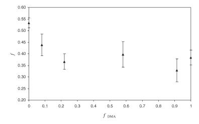
**Figure 6.**Initiator efficiencies ( f) estimated for DMA/ST copolymerization vs. DMA monomer mole fraction. Error bar indicates estimated confidence intervals from parameter fitting.
