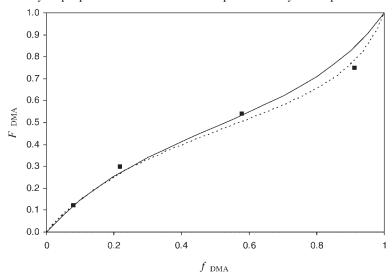
**Figure 3.** DMA polymer composition vs.  $f_{DMA}$  (mole fraction) in the semibatch reactions at 138 °C: experiment ( $\blacksquare$ ); Mayo-Lewis model (-); Lowry Case 1 model with [M]<sub>tot</sub> = 0.5 mol/L (- - -).
