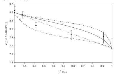
**Figure 5.**Termination rate coefficients for DMA/ST copolymerization vs. DMA monomer mole fraction: estimated values (▲); Walling equation (—); Atherton and North model (— —); Buback simplified model (- - -); Ma model (— - —). Error bar indicates estimated confidence intervals from parameter fitting.
