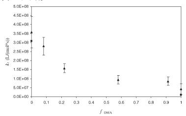
**Figure 4.**Termination rate coefficients for DMA/ST copolymerization vs. DMA monomer fraction, estimated by assuming penultimate propagation ( $\triangle$ ) kinetics. Error bar indicates estimated confidence intervals from parameter fitting. Homopolymerization  $k_t$  values from the literature ( $\blacksquare$ ) are also shown.
