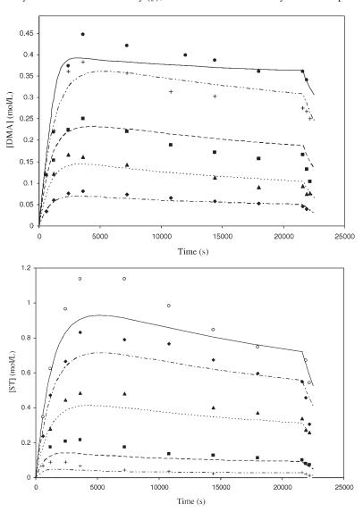
**Figure 7.**[DMA] (top) and [ST] (bottom) semibatch experimental profiles (points) and model predictions (lines): ST homopolymerization (○,——); ST/DMA 75/25 copolymerization (♠,— - —); ST/DMA 50/50 copolymerization (♠,— - -); ST/DMA 25/75 copolymerization (■,— —); ST/DMA 10/90 copolymerization (+,— - - —); DMA homopolymerization (♠,——).
